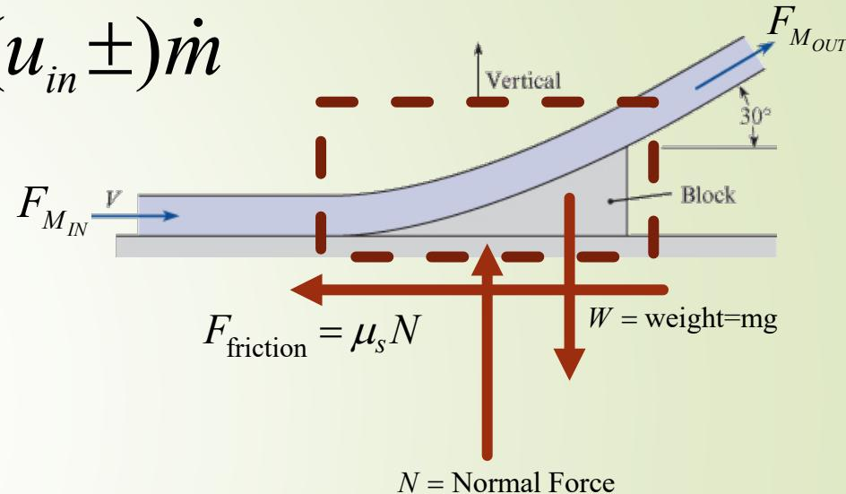
$$\begin{aligned}\dot{m} &= 5 \text{ kg / s} \\ V &= 25 \text{ m / s} \\ \mu_s &= 0.25\end{aligned}$$
